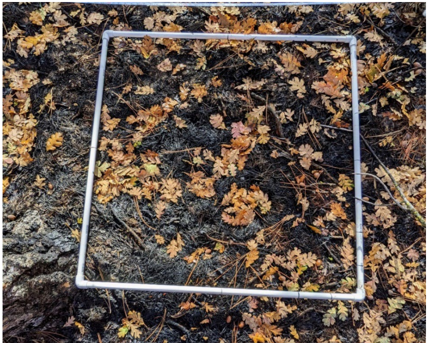
1-m 2 PVC frame used to measure burn severity of substrate and vegetation.
