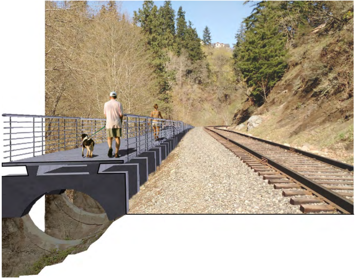
Figure 5: Artist's rendering of an elevated walkway built upon existing concrete saddles (supports for the former pipeline).
